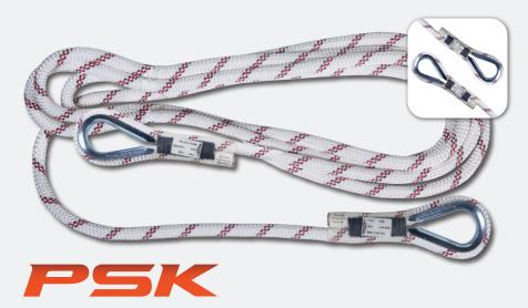
The WestFall Pro PSK Kernmantle - Double Eyed Rope has a 100% polyester, kernmantle construction and meets ANSI Z359.15 NFPA 1983(T). Due to the low elongation of the polyester fiber and customized fiber processing the rope has very low stretch and bounce.
